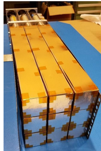
1719 lead glass blocks in 191 supermodules
